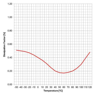
Test Equipment: E4991A or equivalent
