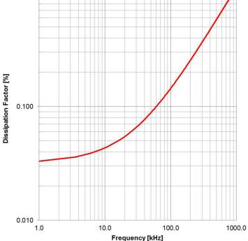
Test Equipment: E4991A or equivalent
