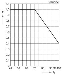
Maximum  $I_{RMS}$  current as function of the ambient temperature:  $I_{RMS}$  ( $T_A$ ) = Factor x  $I_{RMS}$  (70 °C)
